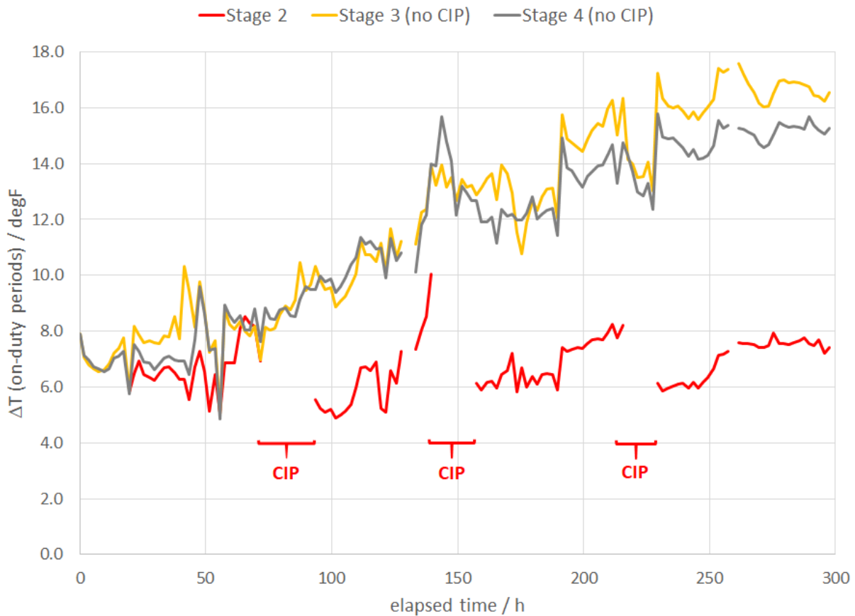
Figure 5 Temperature difference between condenser and boiler in the same stage for three of the regular stages in the Core: Stage 2 (subject to periodic CIP) and Stages 3 and 4 (without CIP capability).
